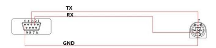
Interface format 1 Communication method RS-232C, 9600bps, No Parity, Data Length: 8 bits; Stop Bit Length: 1 bit STX (02h) Command (3Byte) ETX (03h) 2 Communication format Only 1 command valid per communication. 3 Data format For input commands, only ASCII-compliant all-uppercase alphanumeric characters supported. 4 Replies Acknowledge ACK (06h) CR (0Dh) Data ... Normally ended ... Aborted ACK (06h) ESC (1Bh) No acknowledge NAK (15h)
