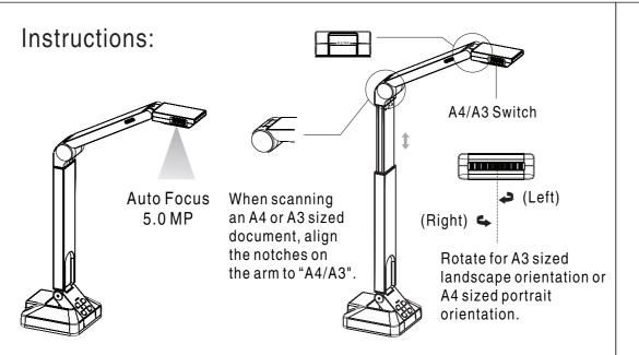
The Camera Switch can be set to A4 or A3.
